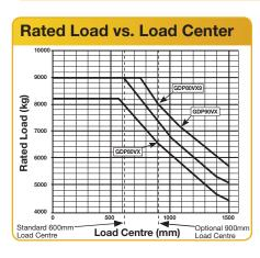
Truck Configuration 2-stage LFL F80 mast at HNHL (5565mm MFH) 80VX6 models.
